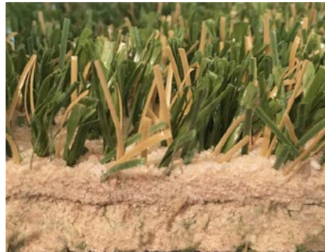
Sand with Polymeric Binder (ArmorFill®) – Flow velocity: 4 to 10 ft/sec
