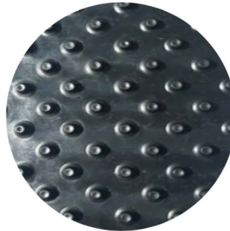
AGRU Super GripNet® (50 or 60 mil) Used for drainage on slopes >3.5H:1V for increased interface friction
